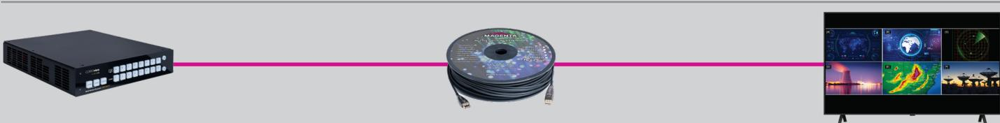
The MG-AOC-66x HDMI 2.0 plug and play cables series supports up to 4K60 4:4:4 with no compression or latency up to 328ft (100m) and is available in UL rated Plenum (CMP), Low Smoke Zero Halogen (LSZH), or with a rugged Armored core, providing the ultimate flexibility.
