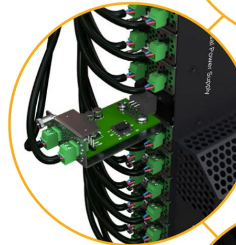
Slide the voltage selector module into the ONErack Spider.
